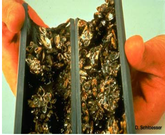
A pipe filled with Zebra Mussels Credit: Don Schloesser, Great Lakes Science Center, National Biological Services
